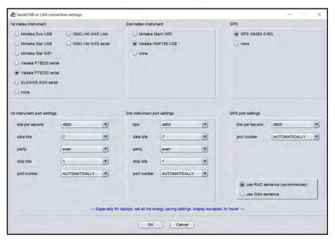
Figure 3: Example serial port settings
