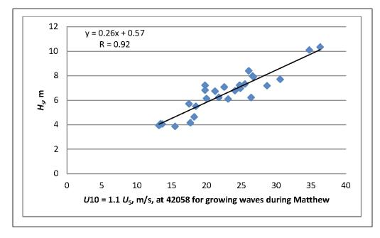
Figure 4. Linear relation between wind speed and significant wave height.
