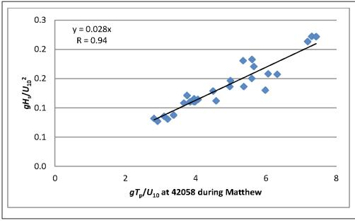
Figure 7. Simplified linear relation between dimensionless wave height and period.
