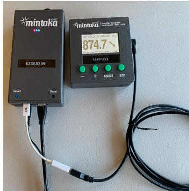
In this case, the STAR is connected via its USB cable to the ENet, and the ENet is connected to the ship's network via an ethernet cable.
