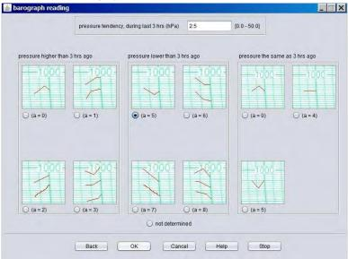
Figure 7: Barograph Reading
