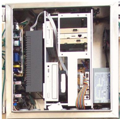
There are two main portions to the SeaKeepers module – one gathers weather data and the other gathers ocean data. The weather portion automatically gathers and records air temperature, relative humidity, barometric pressure, sea surface temperature, and wind speed and direction. Every 3 hours a 10-minute wind speed and direction average is taken, and the measurements are transmitted via a dedicated INMARSAT C transceiver.
